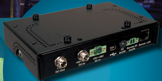
AUPS-B20 VESA 75/100, 9V~36V DC Input 12V DC, 8.3A, 100W Output
