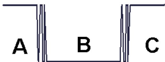
If we just use the read digital input status command to read the signal and we cannot send the command during the B period due to some reasons, then we will lose the key stroke information. However, with the read latched digital input command, we can still get the key stroke information even we are not able to send command in B period. For details of the read latched digital input command, please refer to Sections 2.17 and 3.1.
